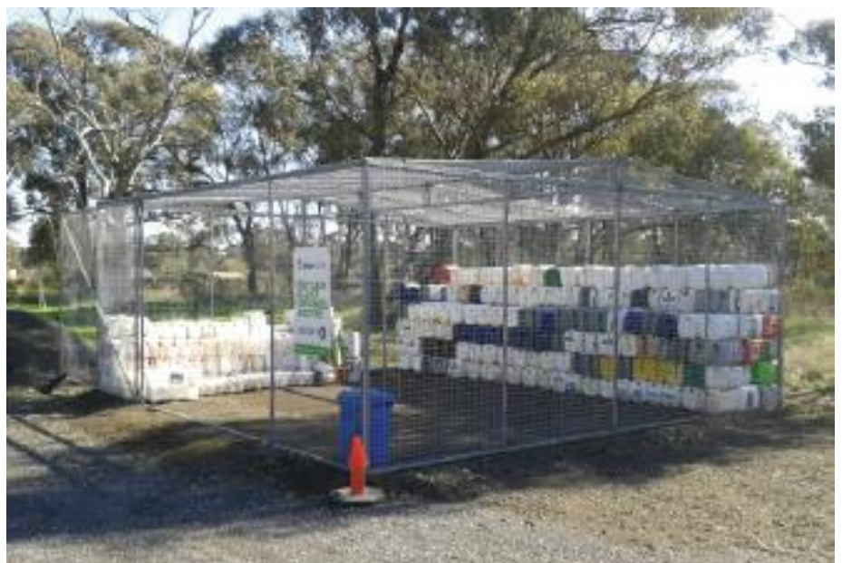
Drums stacked correctly to ensure rain water cannot enter the inspected drums.
